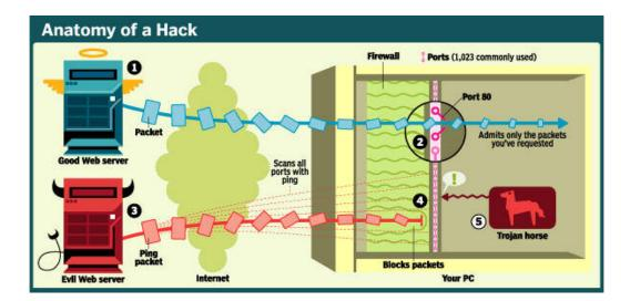
**1.** Web servers send sequences of packets to your computer over the Internet. Each packet has a header that identifies the source and destination computer by IP address and port number.
